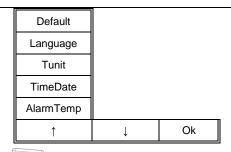
On the sub-menu mode, press to confirm selecting the highlighted option and enter the next sub-menu, press T to exit main-menu operation and return real-time IR mode.
