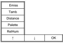
On the sub-menu mode, press to confirm selecting the highlighted option and enter the next sub-menu, press T to exit main menu operation and return to real-time IR mode.
